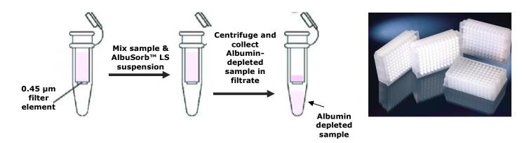
Suspension formats can be processed in single filter-tube assemblies (above) or in microfuge tubes without filter assemblies. Both protocols are adaptable to 96-well formats and automation (right).
